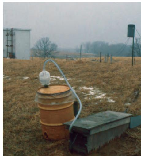
*Surface runoff collection apparatus.*
