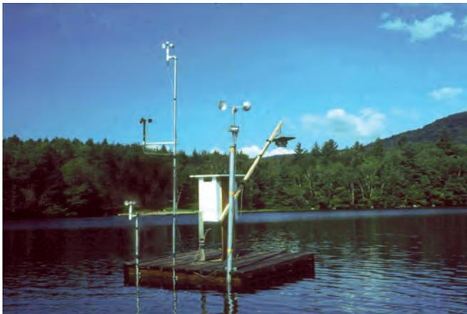
*Instrumentation to measure evaporation from a lake.*
