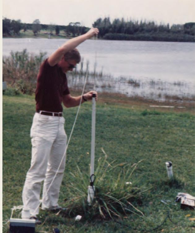
*Performing slug tests to determine aquifer hydraulic conductivity.*
