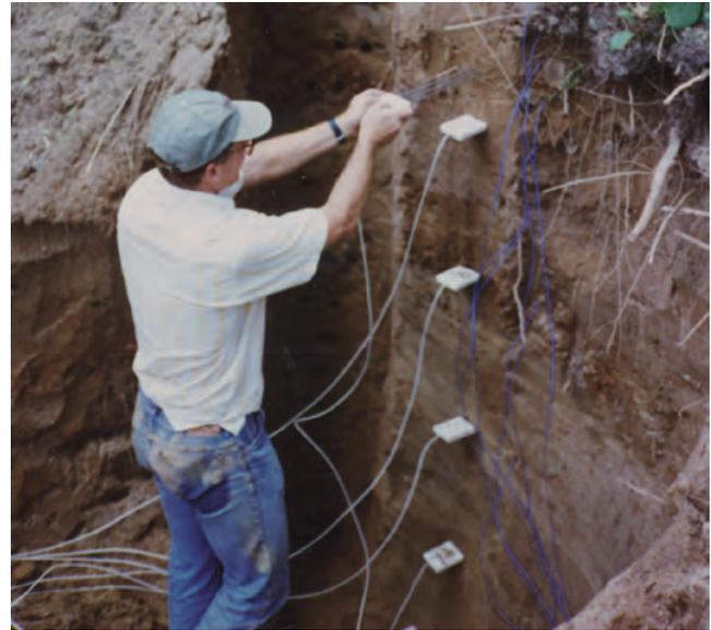
*Installing moisture content sensors through the wall of a trench; the trench was later backfilled.*
