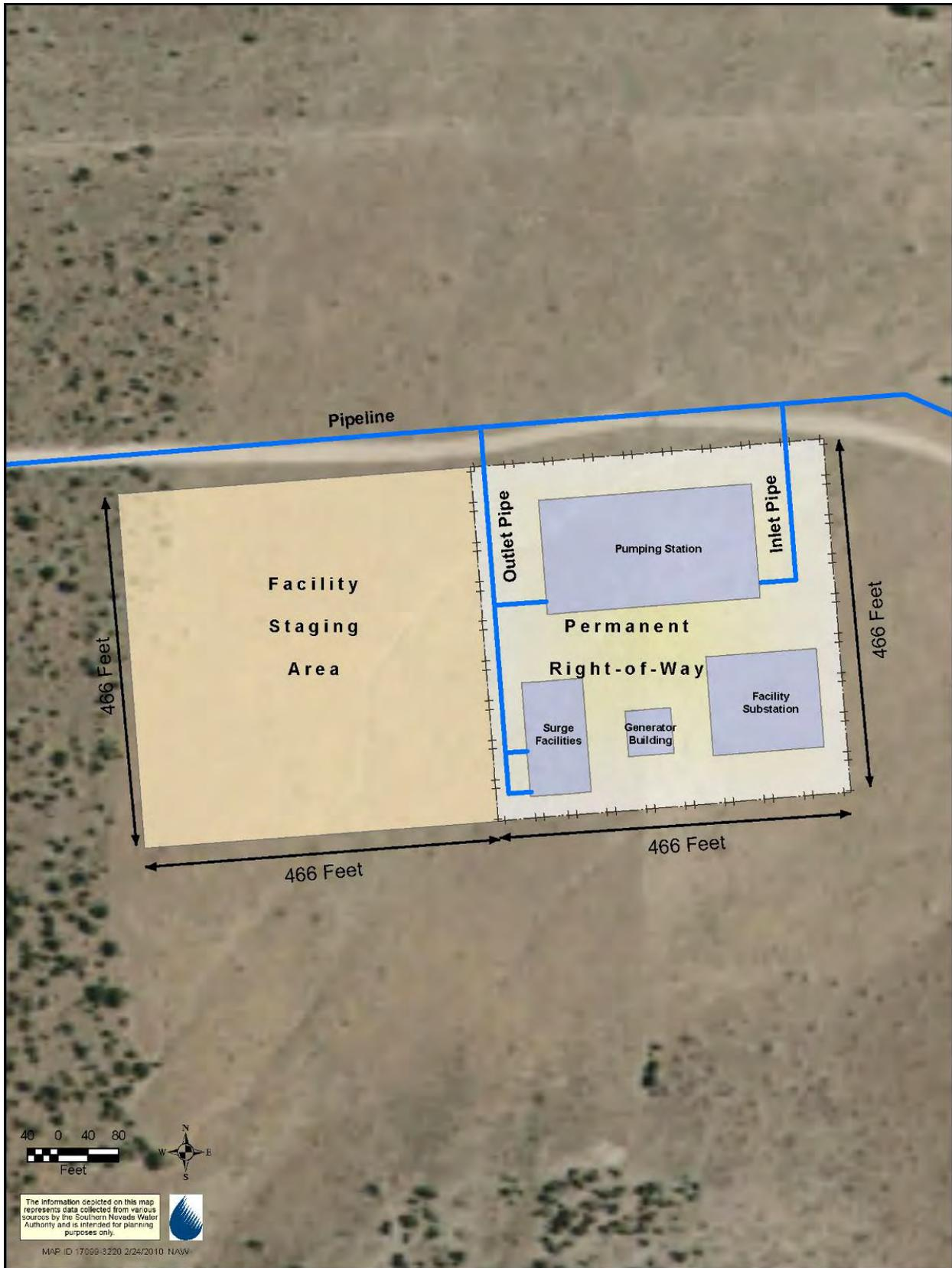
**Figure 2-14 Preliminary Lake Valley Pumping Station Site Plan**
